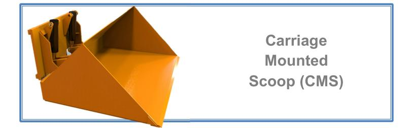
The ideal solution for fork trucks that are dedicated to scooping applications. Hydraulically operated bucket with infinitely controllable discharge rate. Calibrate design with low service requirement. The scoop fits directly onto the truck carriage.
