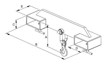
CONTACT Adjustable Fork Mounted Hooks are the most cost effective way of safely hanging a load under the forks of your lift truck. Simply clamps on the forks anywhere along there length.
