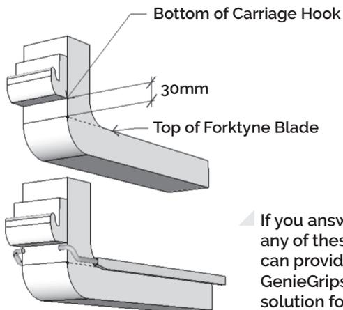
**TYPE B** - is there 20mm clearance between the side of the Carriage Hook and the side of the Forktyne Blade?
